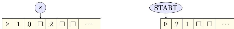
Figure 1: A typical configuration of a Turing machine, and the starting configuration on input 21.
