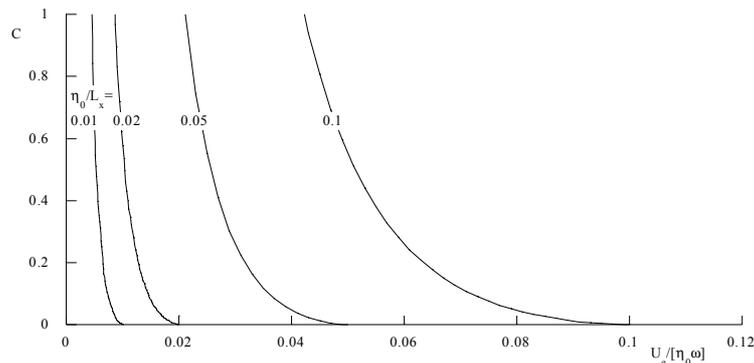
**Figure 6.** Contours of the gradient of the intertidal flat ( $\eta_0/L_x$ ) as a function of the far-field concentration  $C_\infty$  and the magnitude of the threshold velocity for erosion relative to the tidal amplitude and frequency  $U_e/[\eta_0\omega]$ .
