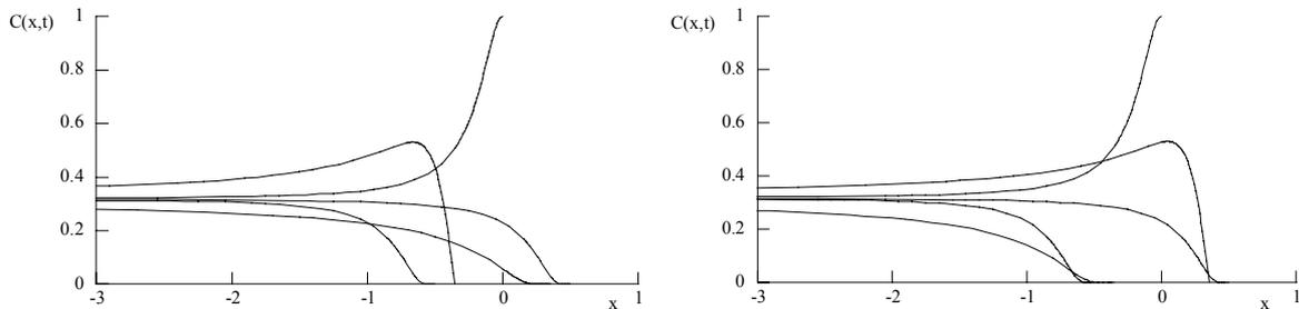
**Figure 3a,b.** The concentration field,  $C(x,t)$ , as a function of  $x$  at temporal intervals of  $\pi/8$ . Figure (a) shows the concentration profiles between high-water ( $t=\pi/8$ ) and low-water ( $t=5\pi/8$ ); figure (b) shows the concentration profiles between low-water ( $t=5\pi/8$ ) and high-water ( $t=9\pi/8$ ). In this plot  $U_c=1/\sqrt{2}$  and  $E=1$ .
