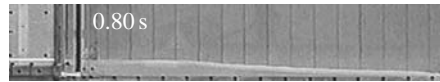
Figure 6. Picture of a particle current formed from an initially fluidized bed of particles described in Roche et al. (2004). The particles are of group A and are released from the reservoir at the left of the picture. The spacing between the background lines is 50 mm.
