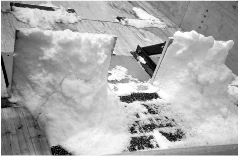
Figure 5. A photograph of wedges left behind the 0.4 m high mounds after an avalanche. Photo: Kristin Martha Hákonardóttir.
