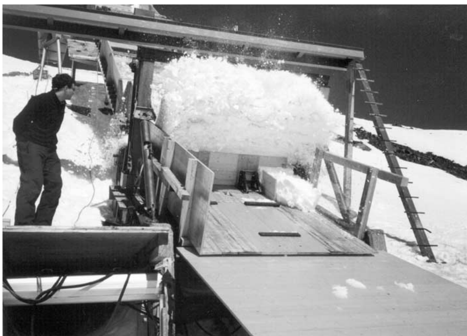
Figure 1. A photograph of an avalanche launched from a 60 cm high dam (and the right hand corner of the dam breaking). Photo: Andrew Hogg.
