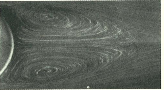
Figure 4.12.8. Streamlines, in an axial plane, of steady flow (from left to right) past a sphere of radius a (from Taneda 1956 b ); R = 2aU/\nu .
