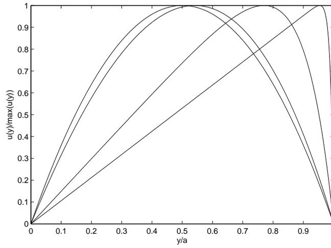
Figure 1: The axial velocity normalised by its maximum,  $u(y)/\max(u(y))$ , as a function of  $y/a$  for  $Re = 0.01, 1, 10, 100$ . (The flow profiles with higher Reynolds numbers are increasing asymmetric.)
