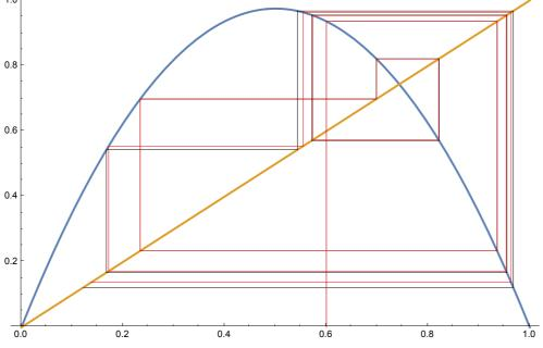
When r = 4 the logistic map is conjugate to the piecewise linear symmetric tent map:  $l_4 \circ g = g \circ t_2$ ,  $t_r = \frac{r}{2}(1 - 2|x|)$  with the bijection  $g(x) = \sin^2(\frac{\pi x}{2})$ . For both maps the image of the map and the attractor are the entire interval, and the dynamics is maximally chaotic, being conjugate to the Bernoulli shift map (see below).
