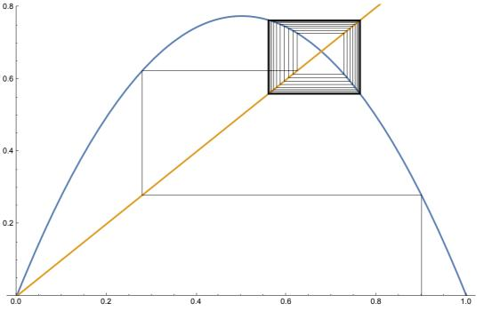
The period doubling bifurcation can be visualised by plotting the orbit of  $l_r^2$ , the second iterate of  $l_r$
