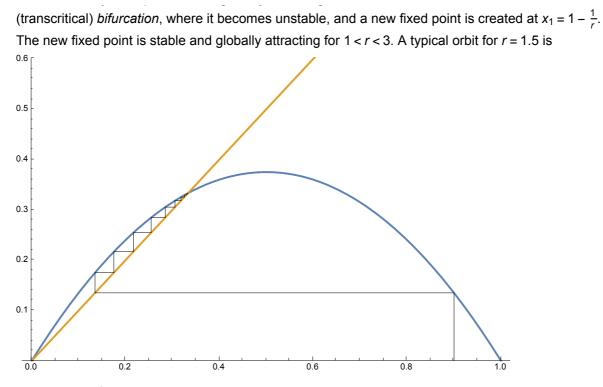
When  $r = r_1 = 3$  another bifurcation occurs when the  $x_1$  fixed point becomes unstable, but this time instead of a new fixed point, a period-2 *periodic orbit* is created  $x_2^{(1,2)} = \frac{r+1+\sqrt{(r-3)(r+1)}}{2r}$ . The orbit is stable if for small  $\delta$
