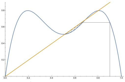
The fixed points of  $l_r^2$  consist of the unstable fixed points 0,  $x_1$  of  $l_r$  and the points of the period-2 orbit  $x_2^{(1,2)}$ , which are stable as fixed points of  $l_r^2$ .
