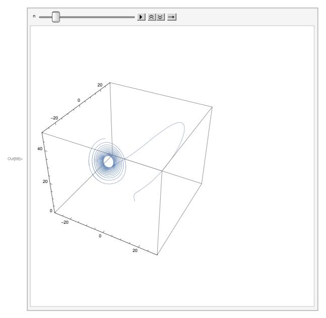
The dynamics can be roughly described as follows: After an initial transient, the orbit is attracted to a butterfly shaped region in the three-dimensional state space. Each wing of the butterfly looks like a slightly curved membrane, but is has a zero-measure transverse component—the attractor is a fractal with dimension slight larger than 2.
