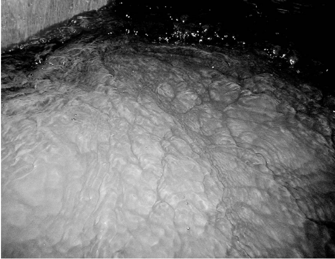
FIGURE 9. The free surface of a turbulent flow. On the surface a network of grooves or ‘scars’ is visible; unpublished photograph by Howell Peregrine.
