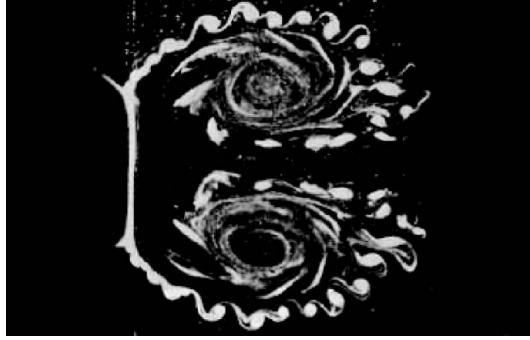
FIGURE 6. The flow around an impulsively started flat plate (Taneda 1987), at a Reynolds number of 3857.
