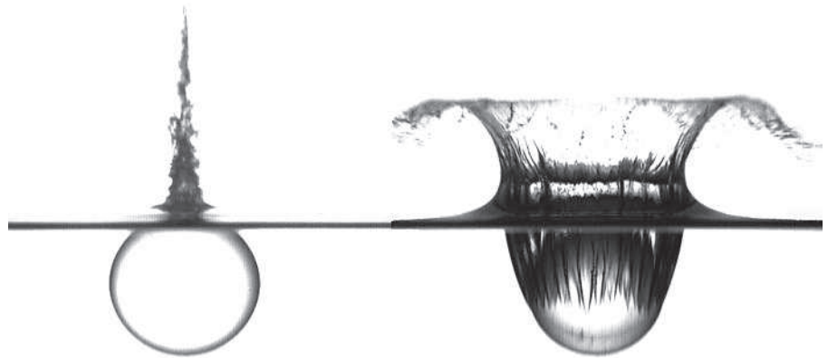
Figure 1 From no splash to a large splash. As the two spheres strike the water at the same velocity, the only difference between the two cases is the surface treatment. (Image courtesy of the authors of ref. 1.)
