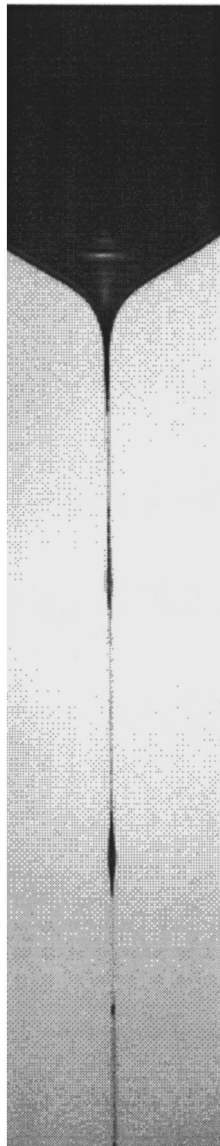
FIG. 19. The same experiment as in Fig. 18, but with a fluid of higher viscosity, ( \mathcal{L}_v=2 mm, t_v=12.8 ms, series GLY3 of Kowalewski, 1996). The height of the frame corresponds to 2 mm. Just before breakup, the thin thread has become unstable and produced several “bumps.” The moment of breakup shows irregular breakup at several places.
