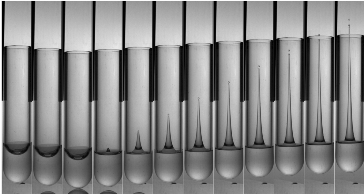
Figure 73. Axial impact of a cylindrical tube falling under gravity and filled with a liquid wetting the tube wall. Following the impact on a rigid floor, the curvature of the spherical meniscus initially fixed by the tube radius reverses violently, a prelude to the birth of a rapidly ascending jet [426].
