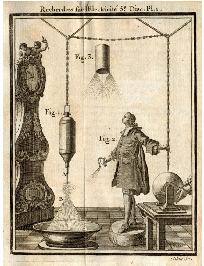
Figure 10. Abbot Nollet himself demonstrating how a water jet disintegrates when it is charged. He notes that (at the location of the letter C) ‘...the main jet spreads and divides itself in several tiny jets’ (from Abbé Nollet (1749) [33]).
