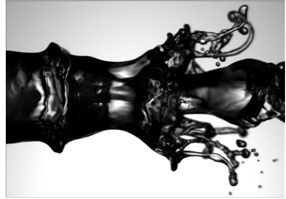
Figure 38. Destabilization of a slow water jet ( h_0 \approx 4 mm) by a fast coaxial air stream [232] ( v_1 = 0.6 m s ^{-1} , v_2 = 35 m s ^{-1} ). The wavelength of the primary axisymmetric undulation is governed by (137).
