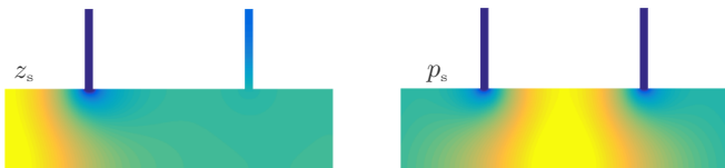
FIG. 10: Real parts of the fields at the zero-transmission ( z_s ) and at the perfect transmission ( p_s ) revealing the shape of the symmetric quasi-trapped mode. Same representation as in figure 7(a) with m=0.2 and 8, respectively
