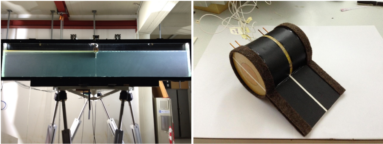
Figure 1: Left: tank mounted on the 6-DOF MISTRAL Hexapode excitation mechanism. Right: boom model and pressure sensors.
