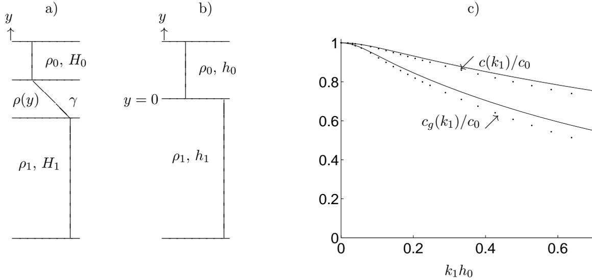
Figure 1: a) Sketch of theoretical three-layer fluid. b) Two-layer fluid. c) Wave phase speed  $c(k_1)$  and group velocity  $c_g(k_1)$ , both normalized by the linear long wave speed of the respective density profiles. Two-layer configuration with  $h_1/h_0 = 18$  (solid line) and three-layer configuration with  $H_1/H_0 = 27.5$ ,  $\gamma/H_0 = 1$  (dotted line).
