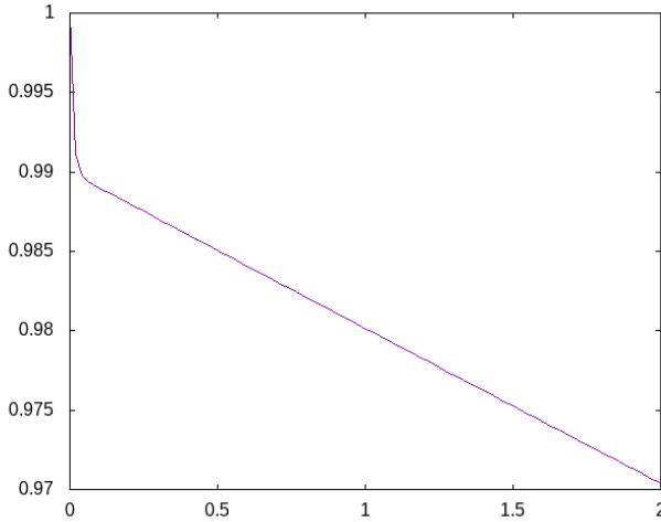
Note that the first term is rapidly decaying and the second term is slowly decaying. Going further, application of the initial condition would give  $A = -\omega^2/(4\gamma^2 - \omega^2)$ ,  $B = 4\gamma^2/(4\gamma^2 - \omega^2)$ . Then  $A$  would be small and  $B$  would be nearly equal to 1. This is interesting, since it shows that there is a rapid decay by a small amount for short times, and then a slow decay over the remaining displacement over longer times. See figure.]
