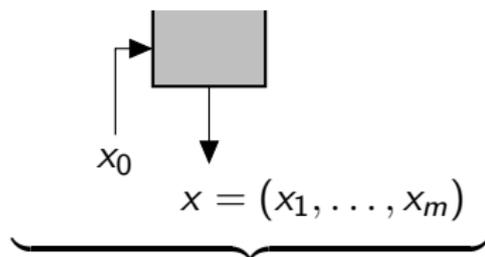
$$\left. \begin{array}{l} \text{Observables} \\ \text{Observations} \end{array} \right\} \begin{array}{l} y_j = g_j(x_0, x_1, \dots, x_m) \\ y_j^{\text{obs}} \text{ (measured values)} \end{array} \quad j = 1, \dots, n$$
